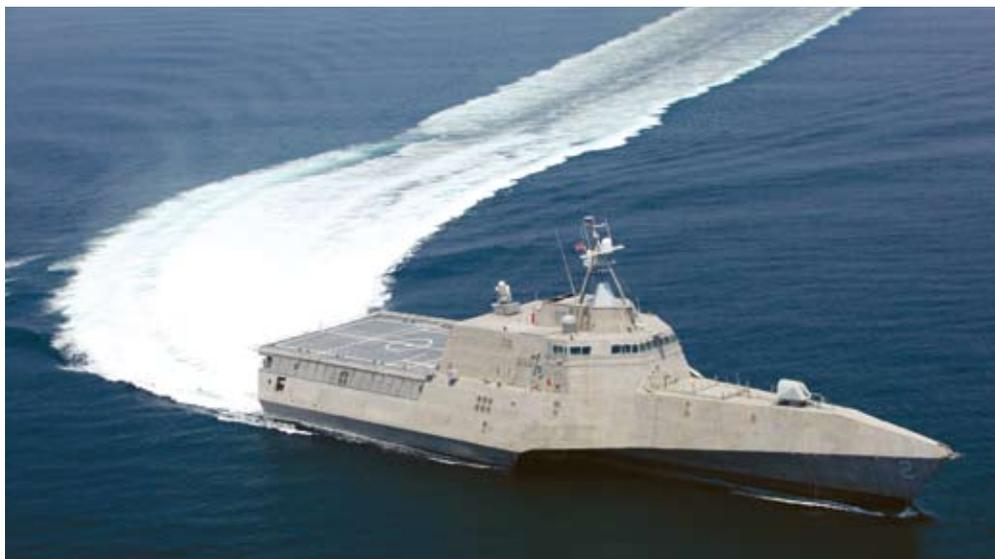
**COMPETING DESIGN ALTERNATIVES** General Dynamics' USS *Independence* (LCS-2, above) is a trimaran based on an Australian ferry; Lockheed Martin's *Freedom* (right), here passing under Montreal's Pont Jacques-Cartier en route to the Old Port, is a semi-planing monohull developed from the *Destrier* commercial vessel. Both support mission modules.
